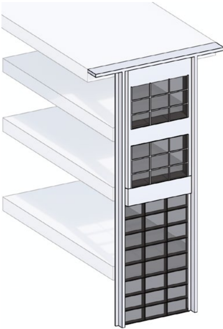
Bay Window Module at Upper Levels
