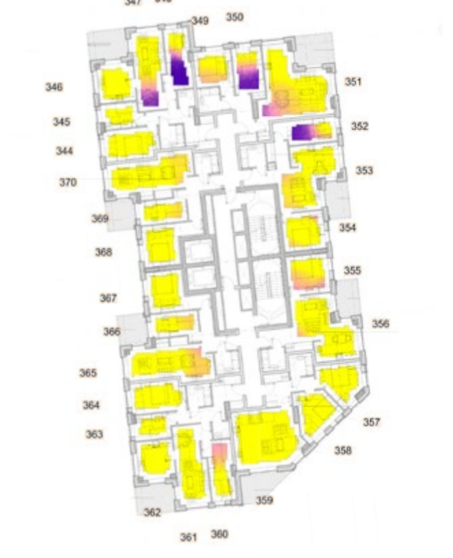
Example daylight analysis from daylighting consultant
