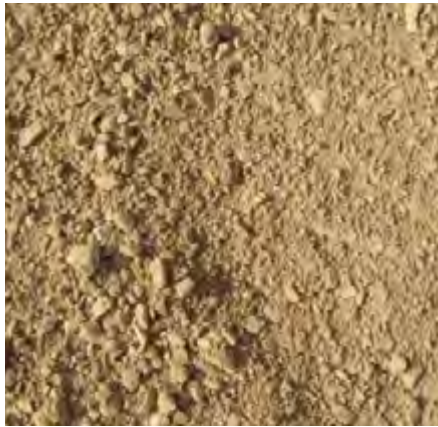
Stabilisé (bound gravel) Pathways in Podium Gardens
