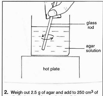
Weigh out 2.5 g of agar and add to 250 cm<sup>3</sup> of distilled water. Heat and stir until the agar dissolves
