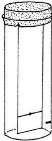
7. Slot the TLC strip into a slit in the cork and put it into an empty tube. Mark the tube below the level of the spot. Remove the TLC strip.
