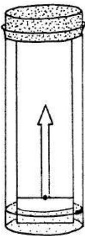
8. Add running solvent to the mark. Put the TLC strip back in the tube. Make sure that it does not touch the sides of the tube. Watch the chromatogram develop.
