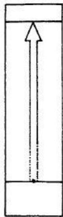
9. After about 4 minutes remove the strip and immediately use a pencil to mark the solvent front.
