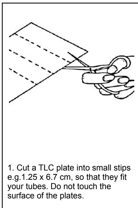
1. Cut a TLC plate into small strips e.g. 1.25 x 6.7 cm, so that they fit your tubes. Do not touch the surface of the plates.
