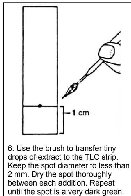
6. Use the brush to transfer tiny drops of extract to the TLC strip. Keep the spot diameter to less than 2 mm. Dry the spot thoroughly between each addition. Repeat until the spot is a very dark green.
