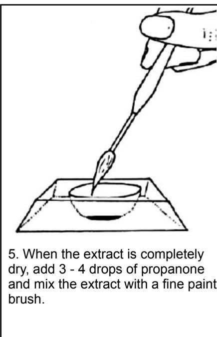
5. When the extract is completely dry, add 3 - 4 drops of propanone and mix the extract with a fine paint brush.
