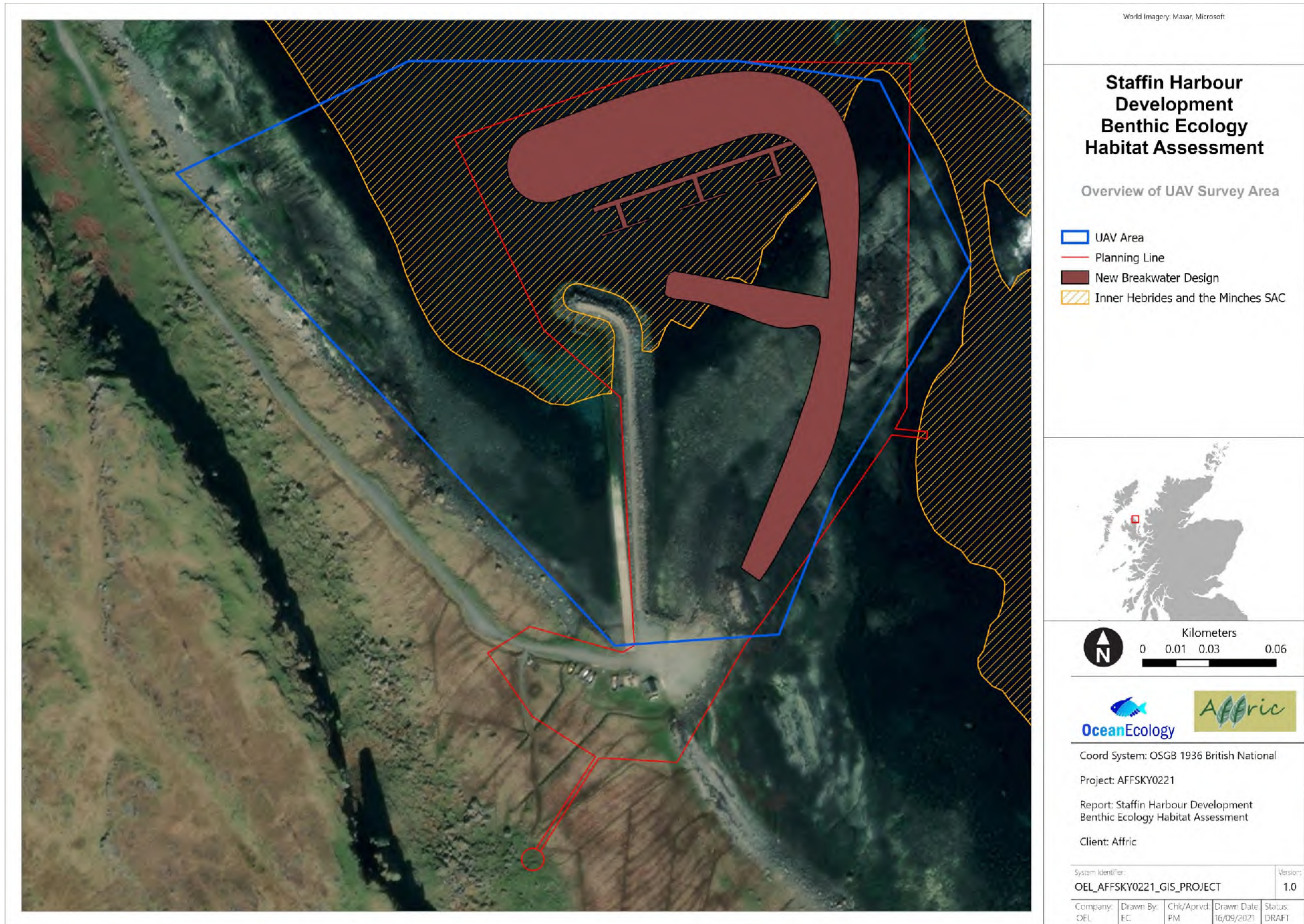
Figure 2 Overview of the Staffin Harbour survey area covered by the UAV flight and new slipway and breakwater designs.
