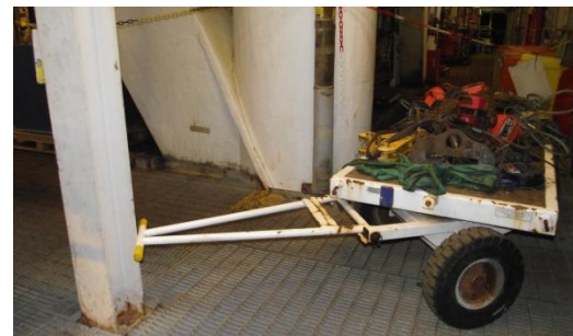
Barrow loaded with rigging gear, Image demonstrates the barrow handle in collision with the H beam
