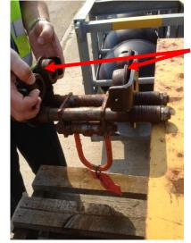
Beam Trolley was incorrectly sized for the gantry beam (the wheel flanges were set approximately 11mm wider than they should have been):
