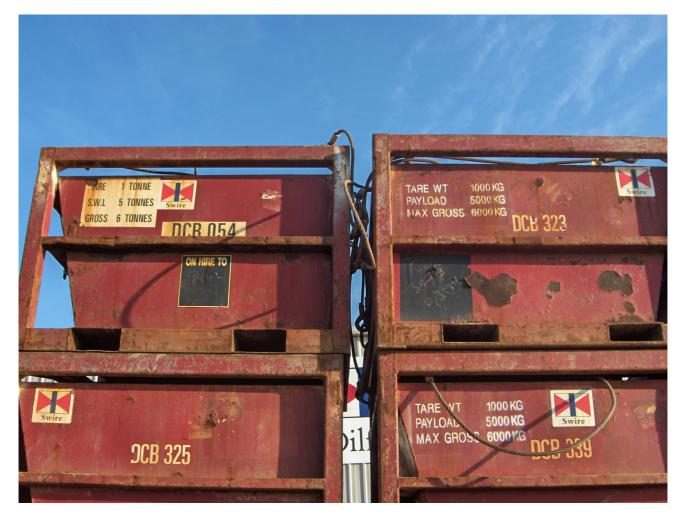
This picture shows the way in which the slings are crushed between units making it difficult for a forklift truck driver to assess if it is snagged or not.
