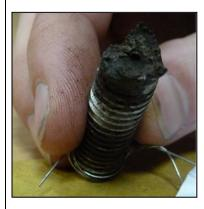
It is concluded that the cap screws failed due to chloride induced stress corrosion cracking, with the final capscrew failing in tensile overload due to the pressure force exerted on the trunnion during pressure equalisation across the valve. The total failure of the trunnion cap screws allowed the valve trunnion to be projected under line pressure from the valve.
