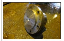
The investigation of the valve found that the six of six trunnion fixing cap screws remained screwed into the valve body but all cap screw heads had separated from the cap screw (at the shoulder). Five out of the six cap screw heads were recovered from the deck within a ten metre radius of the valve.
