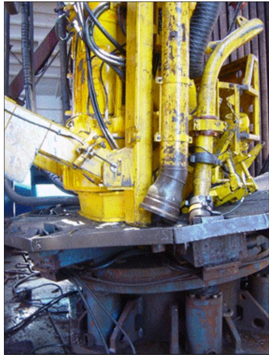
Top drive impacted on riser gimbal at rig floor
