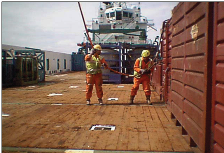
Posed photograph showing typical activities while connecting/disconnecting a container
