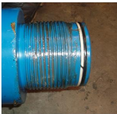
"O" ring and back up in springsele groove
