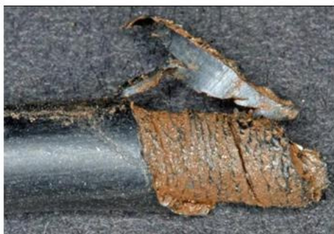
Seal damage due to inadequate support
