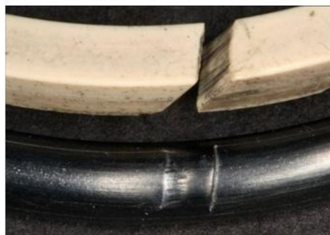
Seal damage due to inadequate support
