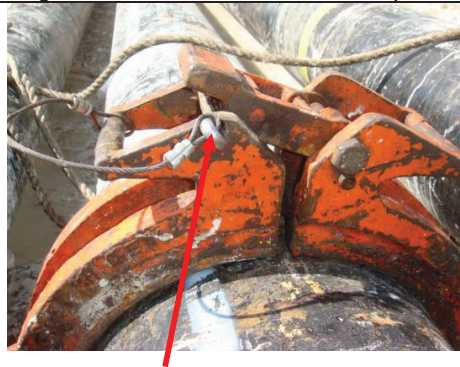
Recreation: Note the latch partially closed with pin incorrectly inserted.
