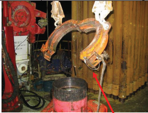
Elevators after the incident. Note the safety pin still in the elevators.
