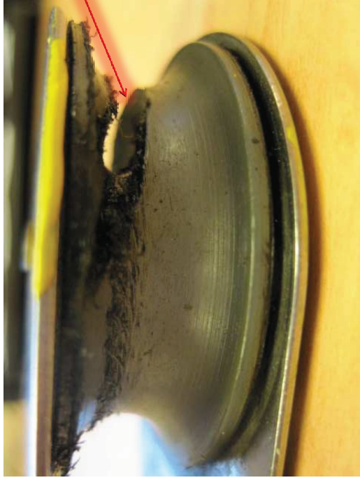
Damage to sheave from Small diameter cable cutting through plastic
