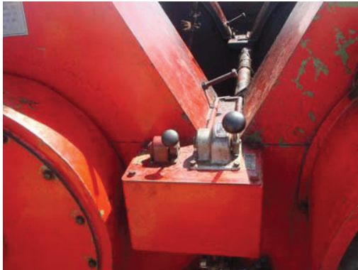
Location of shut down lever and clutch
