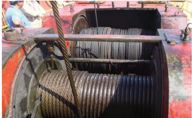
View of drawworks drum and sand-line drum
