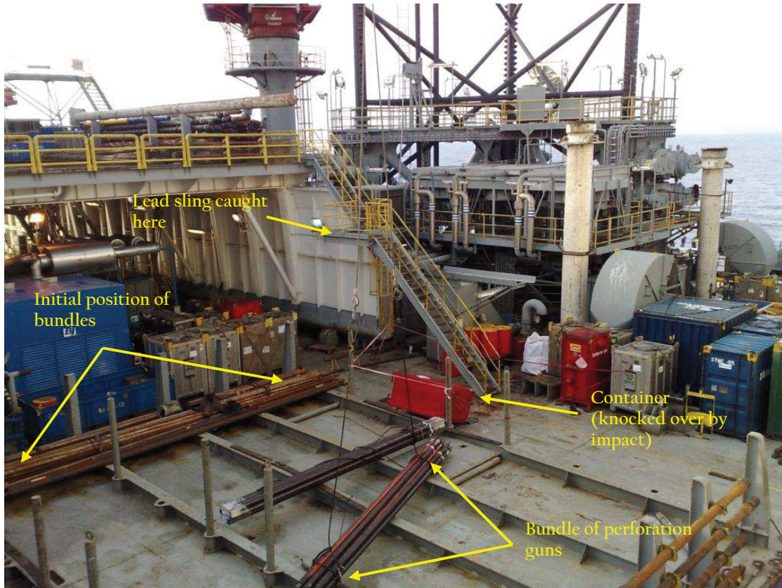
Overhead View of Main Deck, showing location of items related to the incident.
