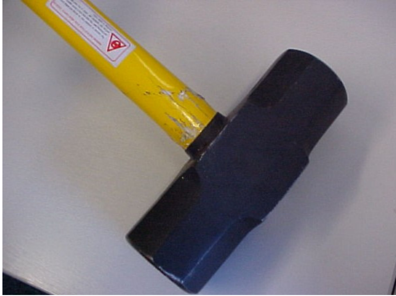
Fibreglass shaft cracked near head of hammer
