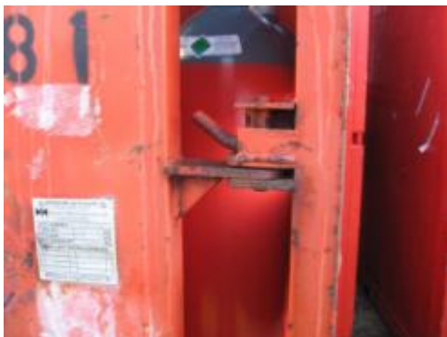
Pin in correct closed position
