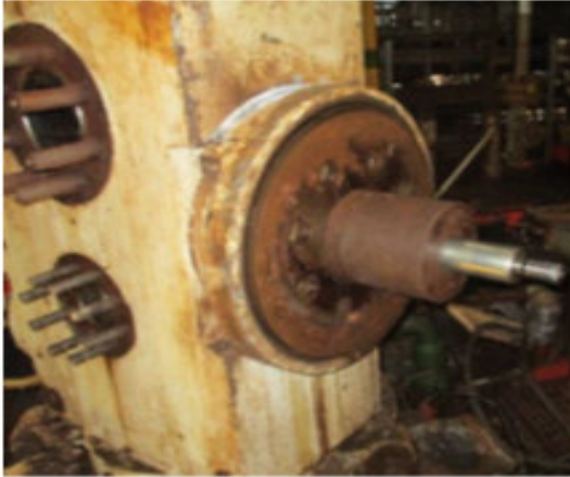
Photograph of tree without volute spring, cover and retaining nut offshore post incident.
