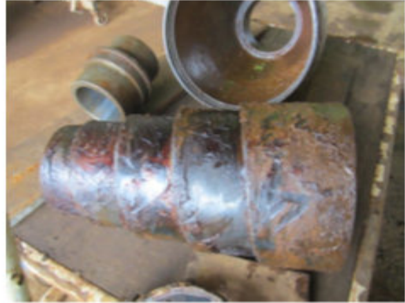
Photograph of Volute Spring and Housing (right rear) offshore post incident.
