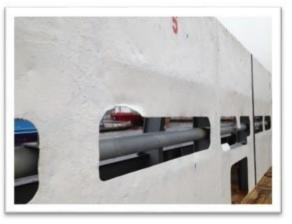
As a result, anti snag bars were fitted to all safe havens and the vessels top rails were highlighted.
