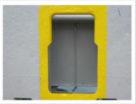
All term contracted PSVs are required to have their cargo top rails marked to highlight potential cargo snagging areas which may be hidden from the crane operator's view.
