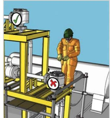
They attempted to remove the bolts from the live-side of the valve, but the high pressure in the vessel prevented the bolts from releasing. Instead they removed all of the bolts from the flare-side of the flange. Gas was released as they split the two halves of the flange. They tried to remake the flange but could not as the valve had become misaligned with the pipe.
