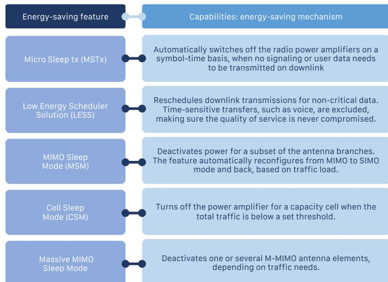
Most of the PSFs provide a set of parameters to control the intensity of their actions, allowing to tune their behavior per cell or node level.
