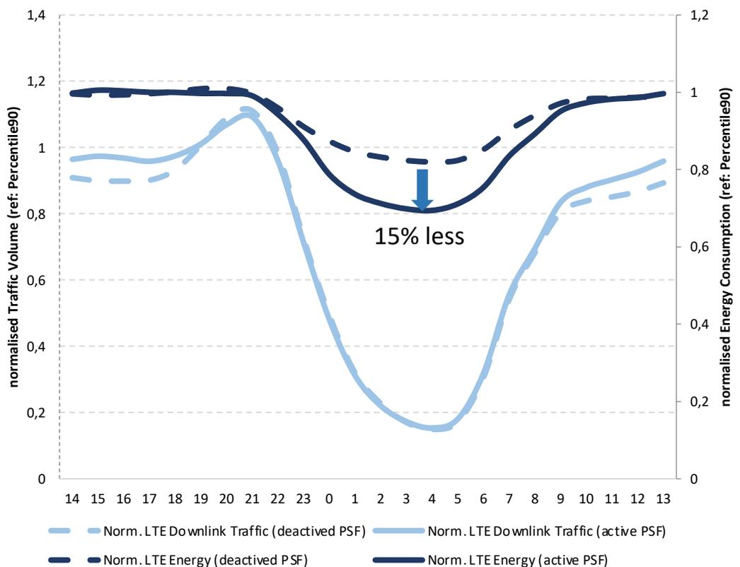
Still, the energy shape is not as abrupt as the traffic reduction. There was (and is) room for more power savings since not all possible power saving features got activated. Considerably higher savings have been achieved in the consecutive iteration phases of AI proposed PSF configurations.
