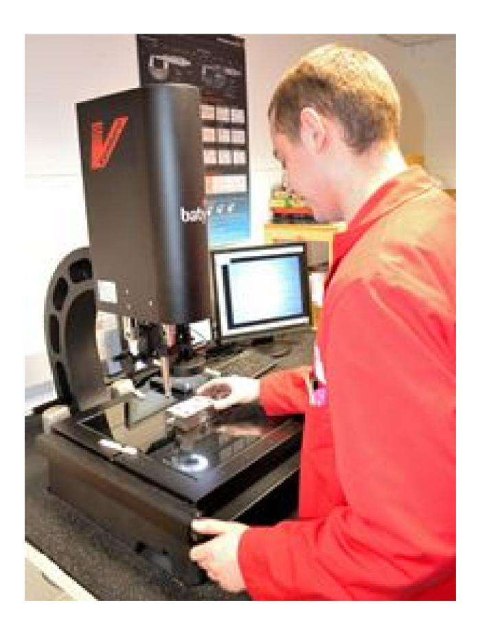
Baty International's highly successful Venture range includes both manual and full CNC systems that cover two standard measuring ranges. The 2510 has a 250mm x 125mm x 165mm X,Y,Z measuring capacity, whilst the 3030, as purchased by Bartorer Precision Engineering has a 300mm x 300mm x 165mm X,Y,Z, capacity.
