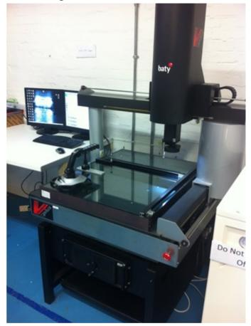
larger measuring range, that could accommodate multiple parts with the added benefit of automatic CNC operation.
