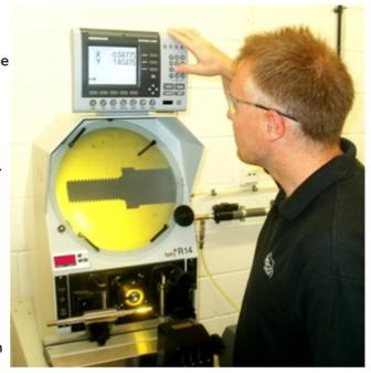
'Shadowgraph' brand is used globally as a generic term for an optical profile projector. Illustrating the continuing popularity of Baty's range of advanced optical profile projectors is the recent sale to Lipco Aerospace Ltd.
