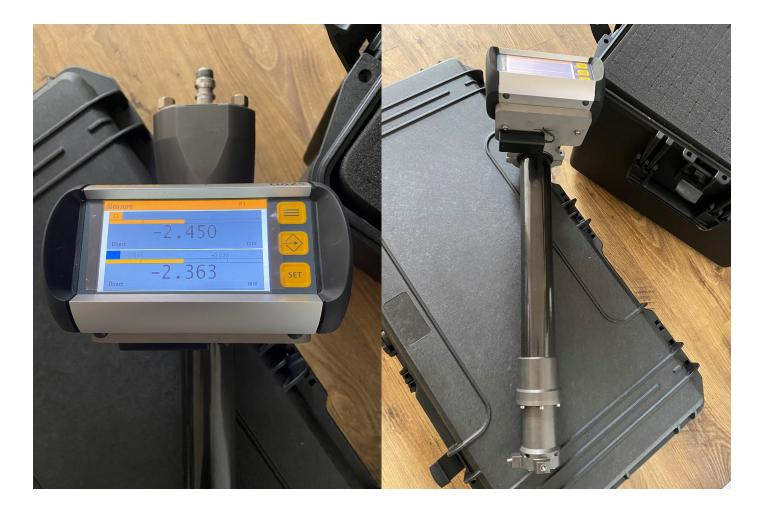
With the team having to repeatedly probe the bore horizontally, making minor adjustments until it met the desired tolerance, it quickly became apparent that having real-time visibility into the part's movement would help speed up the setup.
