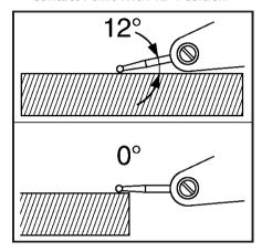
This indicator is designed to provide a true reading when the angle between the contact point and component is 12°. Any configuration of an angle other than 12° needs the displayed value to be corrected. For a position of 0°, the correct value is:
