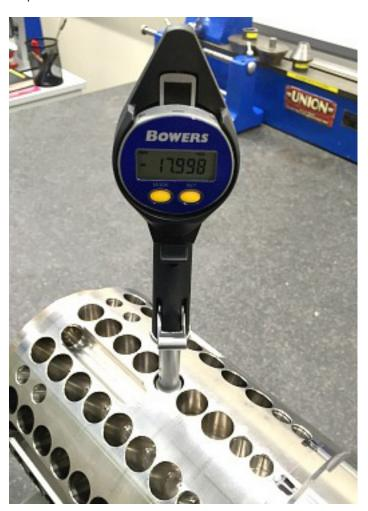
A 'wireless' gauge module is also available, which enables cable free communication with remote data collectors. With a measuring range of 6 – 100mm and simple 2-button operation, the XTL Digital Lever Bore Gauge is excellent for vertical bore measurement and provides fast, accurate measurement.
