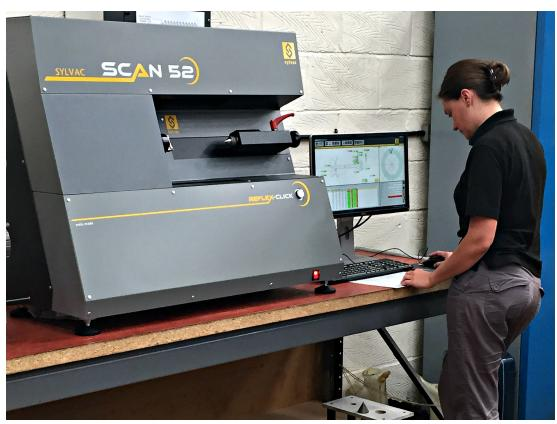
Suitable for first-off part, in-process inspection including Statistical Process Control, sampling, and 100% inspection, the Scan 52 allows Technoset to measure components in the same location as they are machined i.e. on the shop floor.
