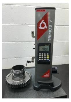
Perfect for use in even the most difficult workshop environments, the Trimos height gauges include simple display units that provide directly accessible functions, depicted with symbols that are easy to understand.
