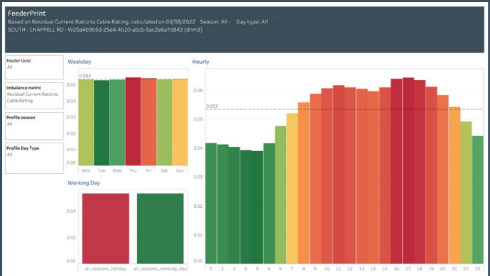
Hourly ranking of imbalance per feeder, creating a feeder 'print' with seasonal day and holiday day variations
