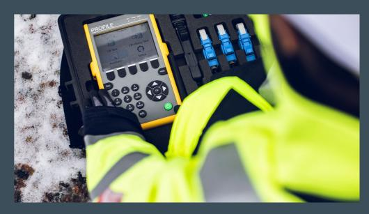
PROFILE P3 provides a unique online insight into the true condition of circuit breakers at all voltages, capturing the vital 'first trip' to show how the breaker would perform in a real-life fault situation. Capturing the first trip gives asset managers insight into the true condition of the circuit breaker, this leads to major benefits;
