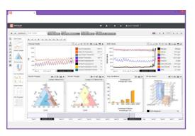
TOTUSPRO Desktop, an optional expert tool for deeper investigation on failure modes, providing customisable widgets and the ability to import offline data archives.
