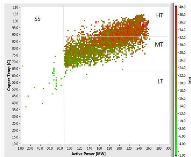
Looking at the beside Map, obtained from a 300 MVA VPI Turbo-Generator, concentrations of red dots are mainly occurring in the HT zone, which means at High Temperature. It is also clear that the red dots are occurring at any power level between 140 and 300 MW, which means that the PD mechanism is not directly dependent on load. As a matter of facts, red dots clearly start to occur above 85°C. This behaviour indicates the **presence of degradation at the semi-conductive**
