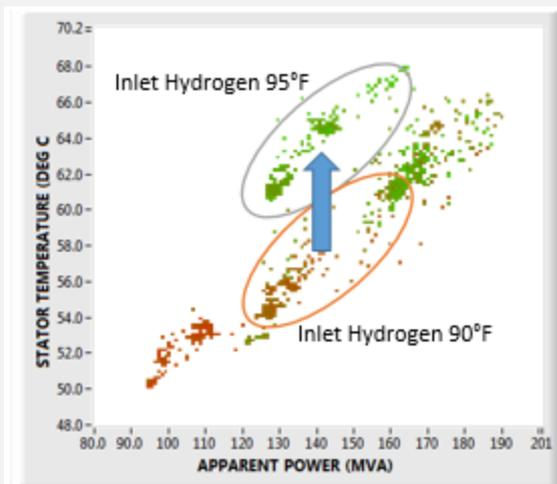
A PD monitoring system applied to a 200 MVA turbo-generator highlighted an inverse relation between PD activity and the machine temperature. Simply acting on the temperature regulator of the cooling hydrogen it was possible to avoid the stator core temperature to decrease below 59°C, defined as the boundary for acceptable PD level from the PDE Map. During the following weeks, the machine was operated in the same load range, but with a different regulation of the inlet hydrogen
