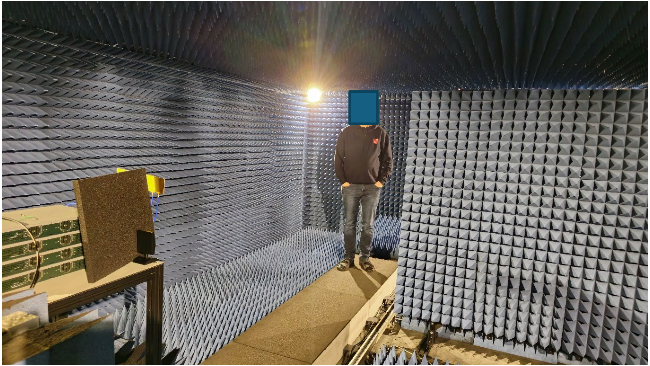
Figure 4-4 Photo of the anechoic chamber ISAC setup with a person in front of the sensing system
