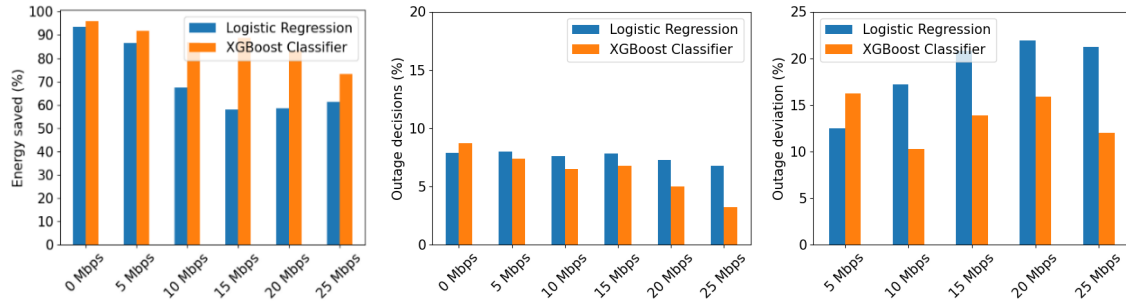
Figure 3-25: 5G Carrier on/off switching – Comparison between Logistic Regression and XGBoost Classifier on policy 1 (outage decisions < 10%)
