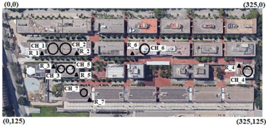
Figure 3-32: Relay-enhanced RAN control - Identified CHs and fixed relay locations to address them.
