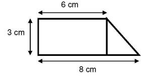
It is easier to split the shape into a rectangle and a triangle. If calculating the area in m<sup>2</sup> it is also useful to convert all distances into m before caclualting the area. The area of a rectangle is equal to its base multiplied by its height.
