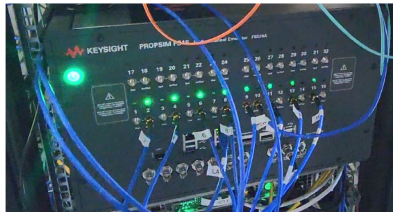
Figure 2-8 Channel emulator – Keysight Prosim
