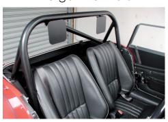
Roll Bars are available for all Morgan models and are suitable for road or competition use. They come in a variety of specifications, including fixed or removable diagonals, seat belt fixings and head rest fixings and so are built to your requirements.
