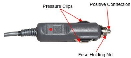
Figure 27 - SeeGull IBflex Scanning Receiver Power Plug
