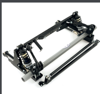
Morgan 5L Suspension System with Spax Dampers supplied & fitted £3,895 + VAT
