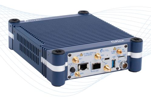
The G*flex*<sup>™</sup> scanning receiver is the next generation of mobile network testing from PCTEL<sup>®</sup>. Designed to support drive testing, walk testing, and government applications for 2G-5G and beyond, the G*flex* sets a new standard for power, portability, and flexibility in a 5G and mmWave capable scanner. A single lightweight G*flex* scanner can collect all the mmWave and sub-8 GHz data you need for drive test, walk test, and government applications in one pass, with one unit.
