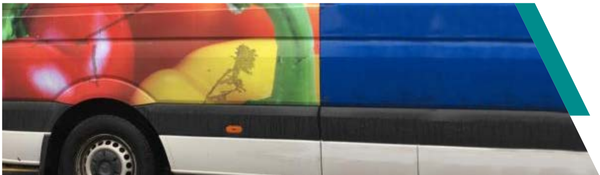
Power-washing too close stripped the laminate, leaving adhesive residue. Dirt stuck to the adhesive, causing dark marks
