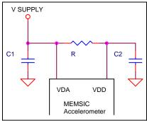
Figure 5: Power Supply Noise Rejection
