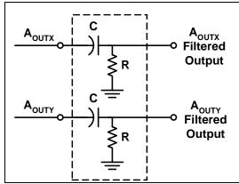
Figure 3: High Pass Filter
