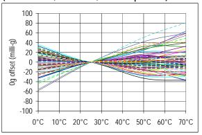
Graph 12. Examples of A<sub>OUTY</sub> 0g offset vs. temperature
