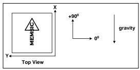
Figure 2: Accelerometer Position Relative to Gravity
