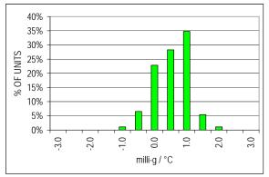
Graph 9. Distribution of A<sub>OUTX</sub> 0g offset over temperature
