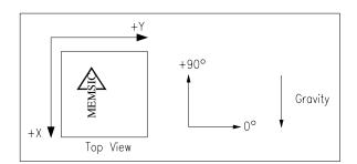
Figure 2: Accelerometer Position Relative to Gravity
