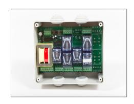
The NECO AC Group Controller is compatible with all single-phase tubular motors.
