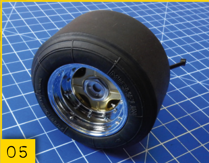
06-05 At last you have united the left front wheel with its suspension.
