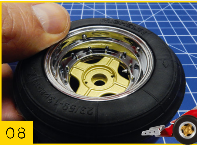
03-08 On both sides of the wheel, check that the lips are married up exactly with the beadlock and the wheel rim. This completes assembly of the first front wheel.
