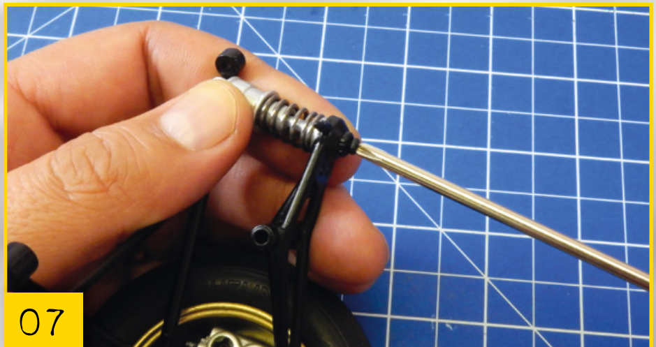
06-08 Insert the hexagonal screw into the slot of the front link, as shown in the illustration.
