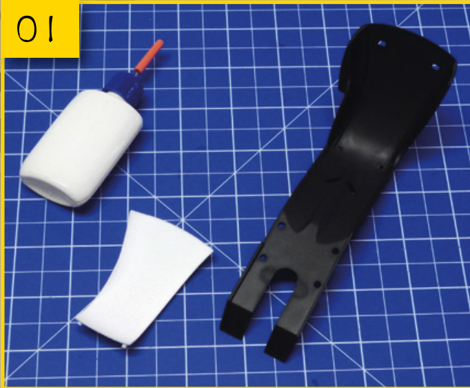
04-01 Begin by assembling the seat: you will need the seat structure, the backrest, and a bottle of plastic glue.
