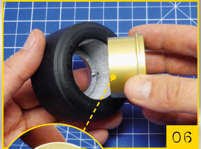
03-06 Insert the wheel rim into the tyre until it connects with the ring. Caution: the holes indicated by the yellow circles in the photo alongside must match up with the interlocking pins of the beadlock.
