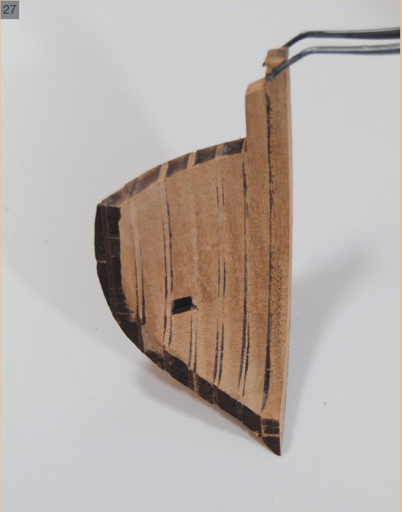
27 Completed hawse piece rear view.
