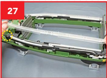
27 Making sure the lower-limit switch and the rails stay in place, lower the right slide rail top into position...
