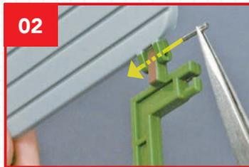
**02** Use tweezers to fit a hinge pin, inserting it from the outside and with the ribbed tip left exposed.
