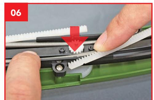
06 Again, fit the spring neatly into the groove beneath the centre gear.
