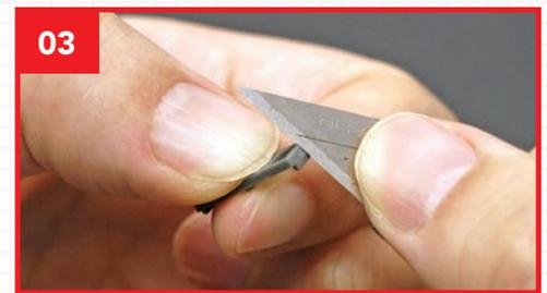
Remove the detail parts supplied on the sprues, then trim any burrs.
