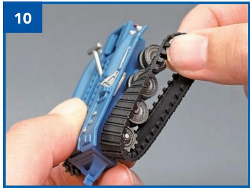
Pull both sets of tracks over the wheels, starting from the drive wheel end.
