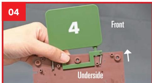
Fit the front hatch assembly to the underside of the floor's front end, via its stay.
