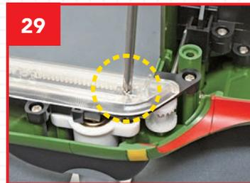
29 Turn a screw lightly into the front hole...
