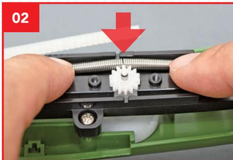
02 Press the spring along the groove, making sure it snaps in past the centre gear.
