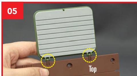
Make sure the hinges are flush with the floor's edge.
