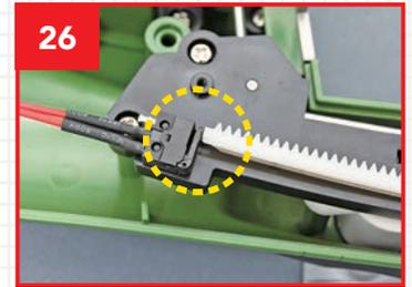
26 The front gear-rail rack should come to rest so it just touches the lower-limit switch, like this.
