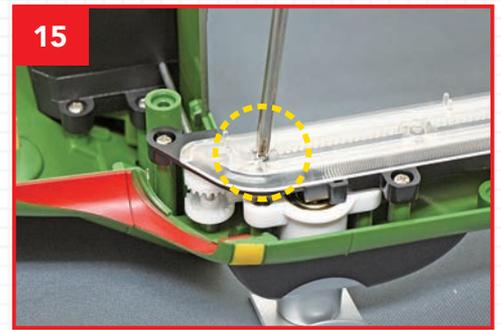
Lightly tighten one of the screws into the front hole.
