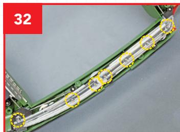
32 ... and then keep going until all these holes are secured. Then fully tighten each one.
