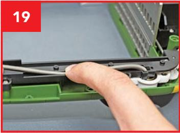
19 Fit the front-right leg spring into its groove, as you did for the left side.
