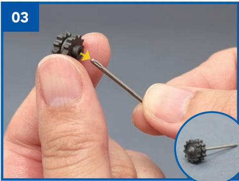
Fit a drive wheel set onto an axle.
